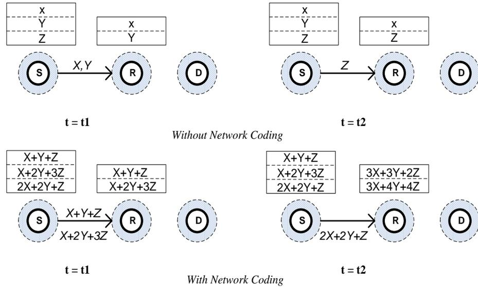
**Figure 5.4:** Improving buffer performance with network coding.
