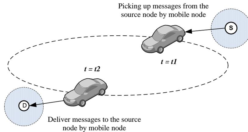
**Figure 3.4:** Message ferrying scheme in active routing protocols.
